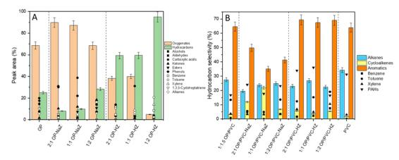
Figure 1. A) Product yield obtained from the catalytic fast pyrolysis of OP over NaZSM-5 (OP-NaZ) and HZSM-5 (OP-HZ) zeolites and B) Hydrocarbon selectivity obtained from catalytic fast co-pyrolysis of 1:1.5 OP/PVC over NaZSM-5 (OP/PVC-NaZ) and HZSM-5 (OP/PVC-HZ) zeolites
