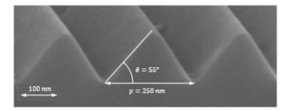
Figure 1. SEM characterization of nanopatterned V-groove silicon substrate.
