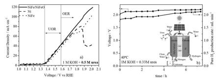
Figure 1. a) Linear sweep voltammetry experiments carried out in a solution of 0.5M urea with 1M potassium hydroxide in half electrochemical cell; b) Proof of concept of hydrogen production via direct PV-AEM coupling
