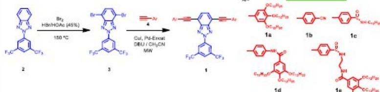
Scheme 1. Synthesis of 2-(3,5-bis(trifluoromethyl)phenyl)-4,7-bis(phenylethynyl)-2H-benzo[d]1,2,3-triazole derivatives (1) by a Sonogashira cross-coupling reaction between 3 and 4.
